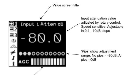
AGC bar graph. Shows gain reduction in 3dB steps. Yellow = less than optimum signal level. Green = optimum signal level Red = overload
