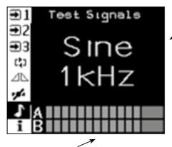
Loop Current bar graph for each channel. Shows Loop output current in 2dB steps from >-20dB to 0dB in green. Red = clipping
