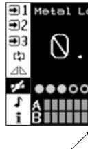
Loop Current bar graph for each channel. Shows Loop output current in 2dB steps from >-20dB to 0dB in green. Red = clipping
