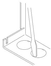
Remove the required knock-outs for cable entry.
