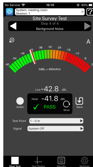
Turn the HLS-2D driver off, save a background noise reading at each test point
