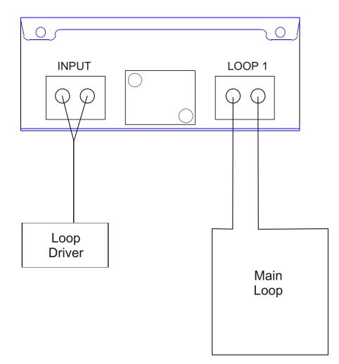
Ensure that the loop terminals are connected in the correct phase where indicated on the loop layout drawing or other documents supplied as part of a special design.
