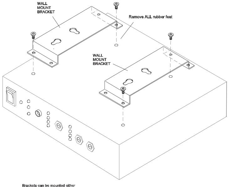
Brackets can be mounted either way round dependant on required equipment orientation. Both brackets must be mounted in the same orientation. Torx T10 sized screw driver is required.
