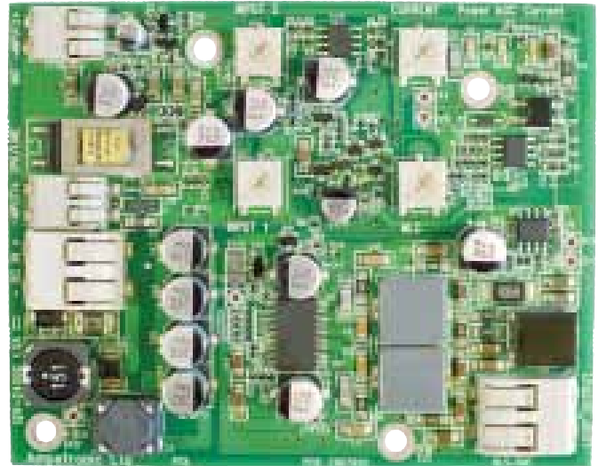
HLS-DM1 Shown at actual 1:1 scale (90.5x72x9mm)
