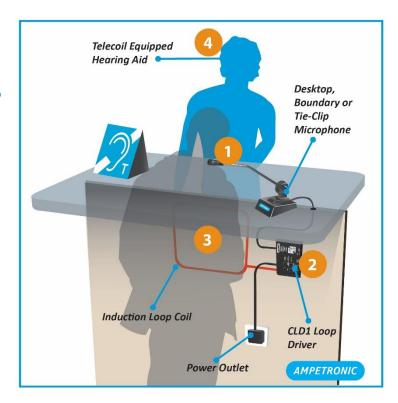
To use the system a hearing impaired customer needs only to switch the hearing aid to the 'T' position. Expensive receivers are not required and users don't suffer the inconvenience of asking for and wearing a headset that marks them out as hard of hearing.
