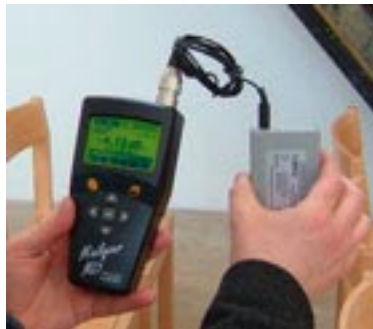
Induction Loop Measurement
