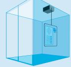
Installation behind a metal panel or metal trim will rarely produce an effective magnetic field with any amplification method. Please contact Ampetronic for detailed guidance on the best installation method for your lift car or industrial environment.
